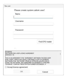
You can search EPD reader port number automatically. Press "Find EPD Reader" button then connect or reconnect reader to USB port. System will identify changes and will provide port number. Search mode will continue 10 seconds or till device is found. You can repeat search. Port number can be entered manually into DosiBase settings.
